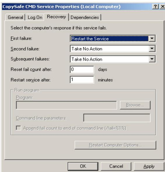
In the **Recovery** tab change the First failure option to Restart the Service.
